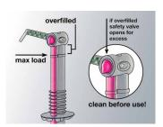
Any paste extruded on the sides of the mixing tip joint must be wiped off before the application in the mouth
