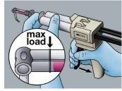
Hold firmly in place while filling. Leave mixing tip in angled position; do not fold open. Do not fill syringe past the maximum fill line.
